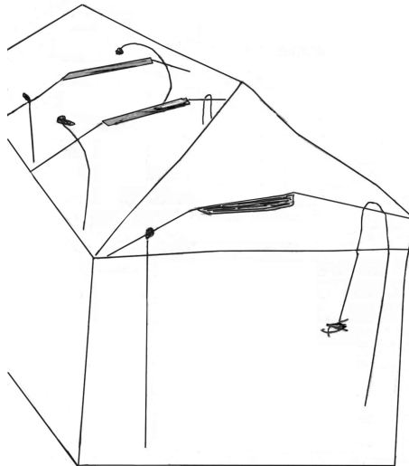
Figure: Sketch showing weighted ropes being thrown over the metal rafters that traversed the width of the hall. 10
